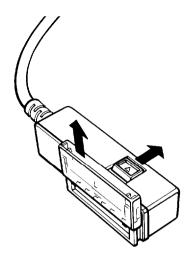
4. Slide this box up into the slots on the connector on the back panel of the computer. Press the connector box up until it snaps into place.
